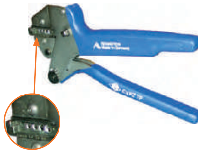
front view showing incorporated crimping dies
